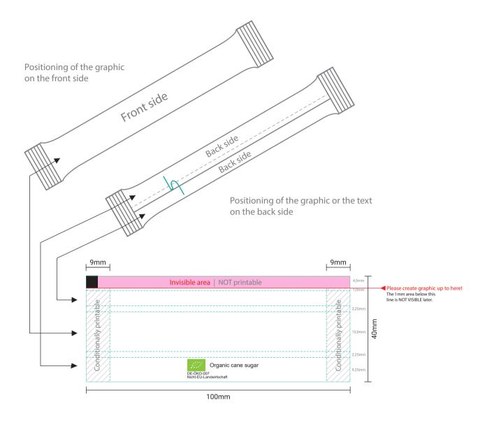
Auxiliary lines (sealing area) + format limitation, can be omitted when creating, these are only used for checking during digital previewing.
